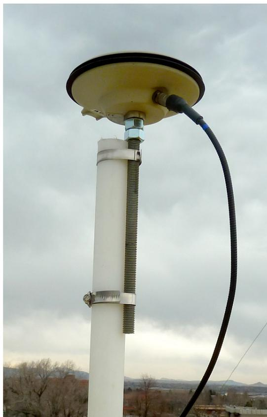
**Fig. 3.** GPS antenna mounted on rooftop location.
